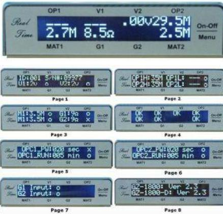
**Main Screen:** Display the real-time measurement value of the resistance and voltage.
